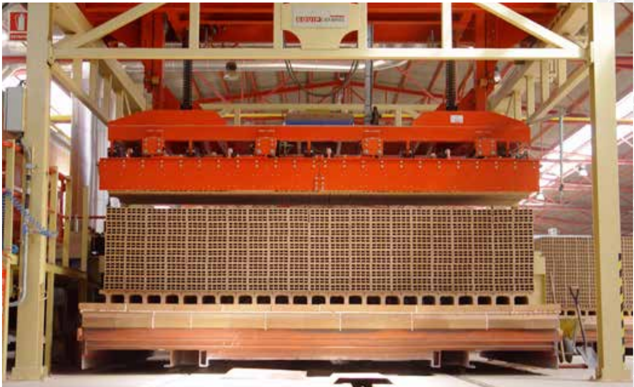
KILN CAR LOADING | CARGA VAGONETAS | CHARGEMENT WAGONS
